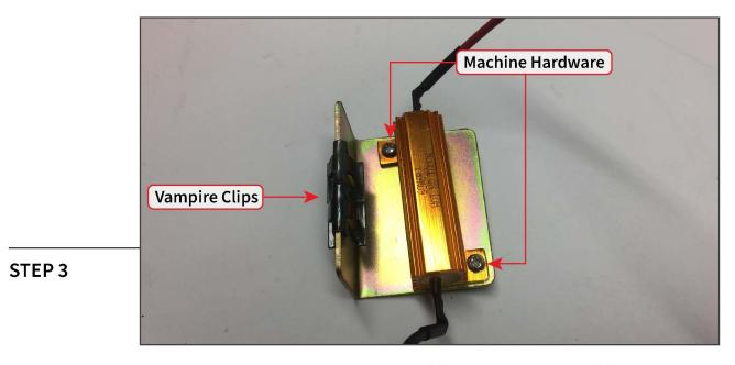
Secure the tail light resistor to the included bracket using (2) machine bolts and (2) machine nuts, tighten until secure.
