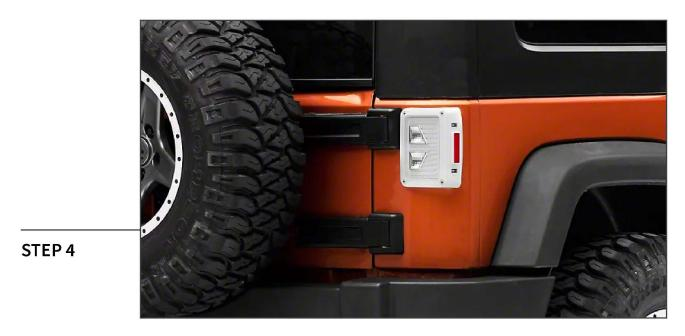
Secure the resistor bracket to the vehicle sheet metal using the vampire clips. Then, plug the tail light into the vehicle wiring harness. Fit the tail light into the vehicle, and secure into place using the original (2) Phillips screws. Tighten the screws evenly until secure.
