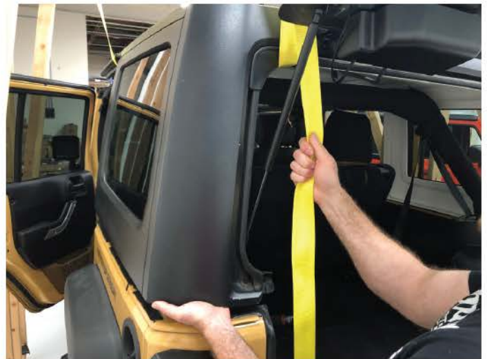
Once you have the top lifted about an inch, grab the bottom edge of the top and lift upward while pulling the strap.
