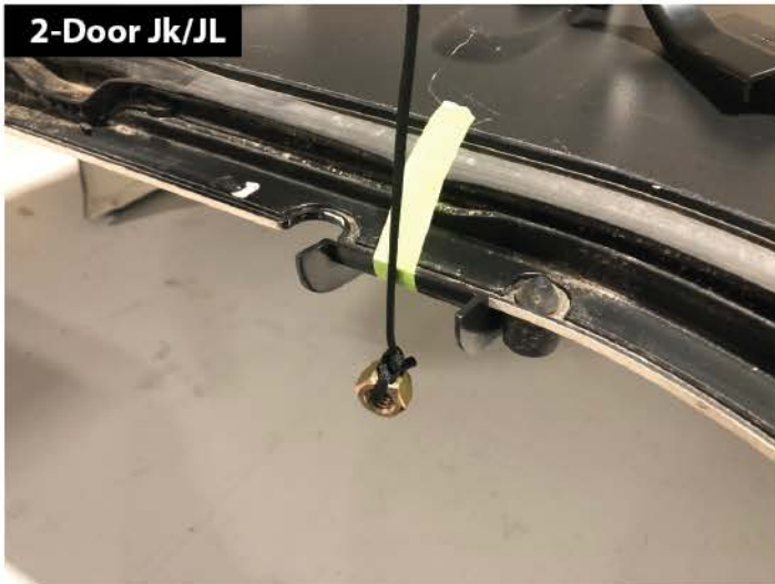
Center plumb line along the edge of the front strap guides, as shown.
