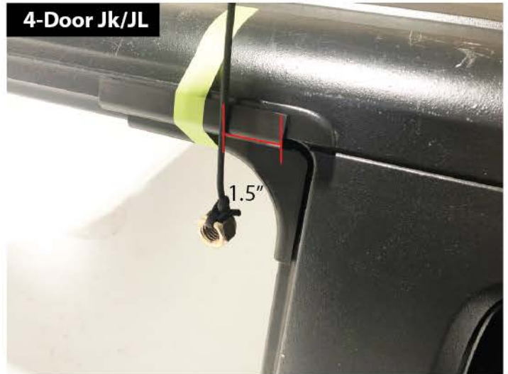
Align plumb line against the outer most edge on the front strap guides, 1.5" from the edge.
