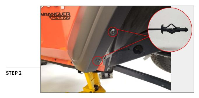
Remove the (2) plastic rivets located above by using a small screw driver and pushing the center of the rivet through. Then, fully remove the rivets from the fender flare.
