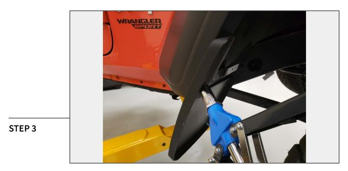
Install the mud guard to the vehicle using the (2) plastic push clips from Step 1. Then using a 1/4" rivet gun and (2) plastic rivets, carefully rivet the side of the mud guard to the factory fender flare.
