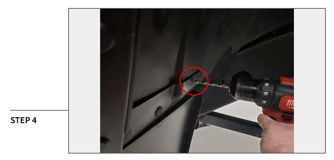
Using a drill & 1/4" drill bit, drill the additional hole into the factory fender liner. Then using a rivet gun and (1) plastic rivet, rivet the inner section of the mud guard to the fender liner.
