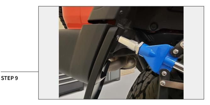
Using a 1/4" rivet gun and (3) supplied plastic rivets, rivet the mud guard to the rear bumper.
