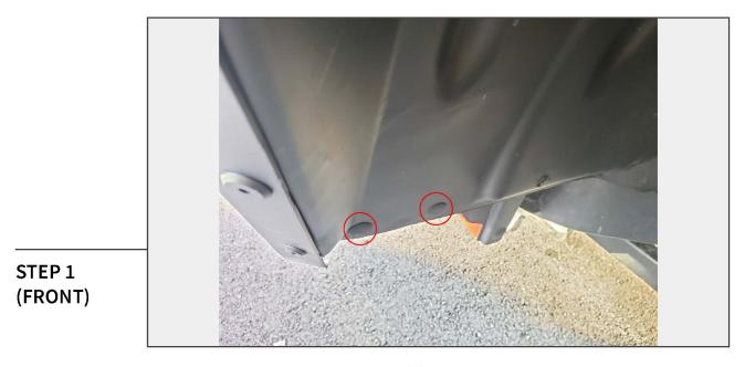
Begin by using a trim panel removal tool, remove the (2) lower push clips securing the back portion of the front fender liner in place.
