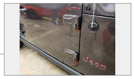
Begin by removing the T-50 Torx nuts on the bottom of the factory door hinges. These will not be reused.
