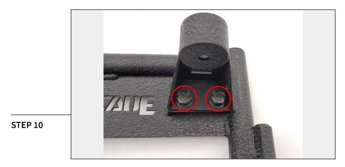
Install the mirror mount to the door using the (2) M10x1.5x20mm bolts, lock washers, and flat washers.
