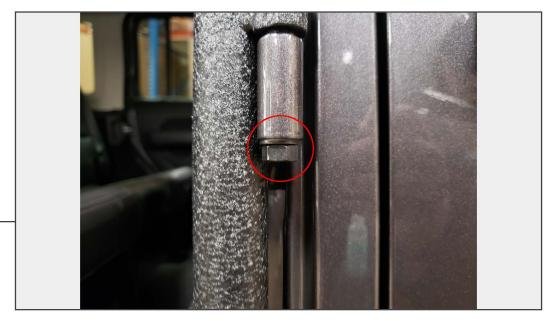
Install the new door, you may need to use a rubber mallet to seat the door all the way onto the hinge. Use the supplied M8 nut and washer to secure the door to the hinge.
