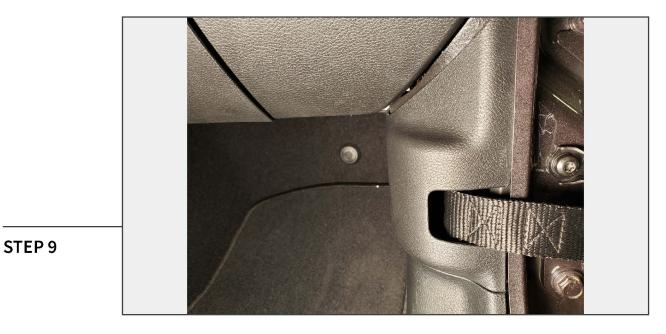
Install the door strap from the new door to the chassis mount. Reinstall the interior trim panel.
