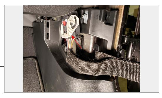
Roll down the windows so that the door is easier to handle while removing it from the vehicle. Unplug the door electrical connector by sliding the red lock, and then folding the white connector latch. Slide the hinge strap off the chassis mount hook.
