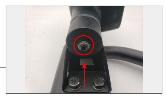
Install the supplied mirror to the mirror mount using the (1) M8x1.25x20mm bolt, flat washer, and lock washer.
