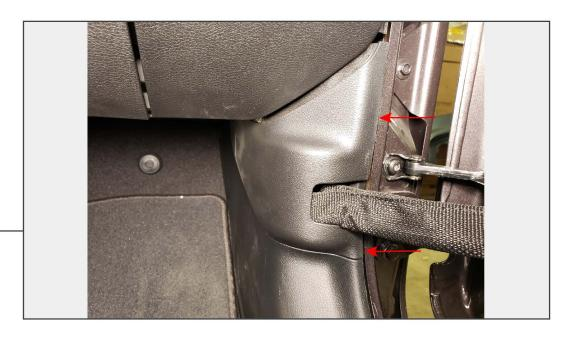
Using a panel removal tool, pry the kick panel away from the vehicle body.
