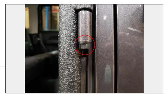
Install the new door to the vehicle hinges, you may need to use a rubber mallet to seat the door all the way onto the hinge. Use the supplied M8 nut and washer to secure the door to the hinge.
