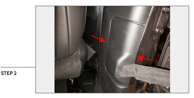
Slide the front seat forward to access the interior trim panel. Using a panel removal tool, pry the panel off. \*\*Note: The panel has indents on the sides, pry from those indents.
