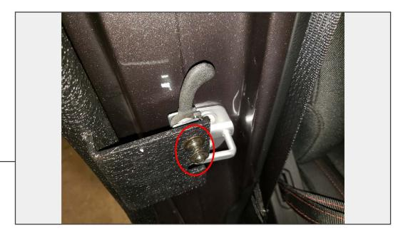
Loosely install the door latch using the M6x25mm screws, flat washers, and lock washers.
