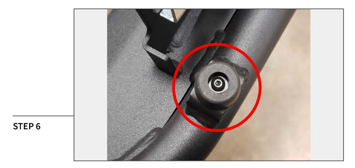
Install the rubber door stopper to the door using the M4x15mm screw, and M4 flat washer.
