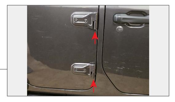
Begin by removing the T-50 Torx nuts on the bottom of the factory door hinges. The nuts will not be reused.
