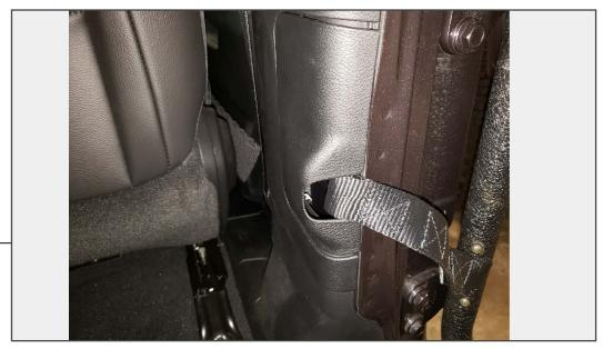
Install the door strap from the Tubular Door to the chassis mount. Re-install the vehicle trim panel.
