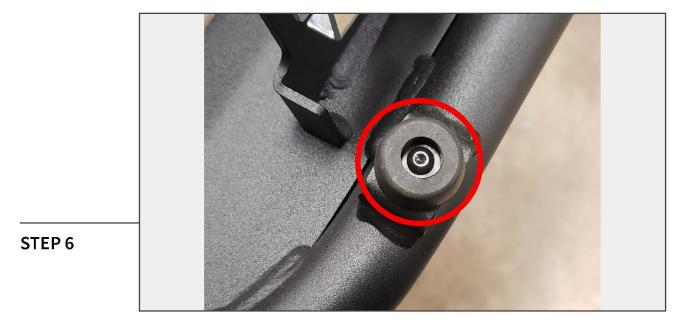
Install the rubber door stopper to the door using the M4x0.7x15mm bolt and M4 flat washer.
