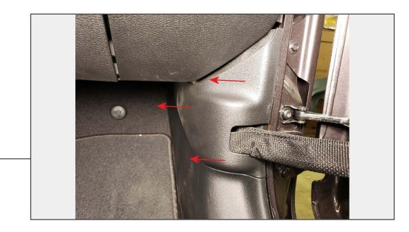
Using a panel removal tool, pry the kick panel from away from the vehicle.
