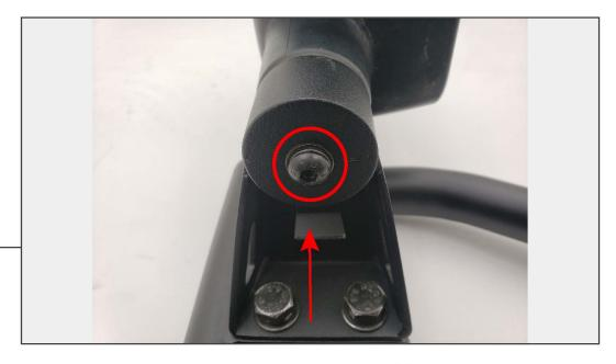
If purchased separately, install the JK mirrors to the mount using the (1) M8x1.25x20mm bolt, flat washer, and lock washer.
