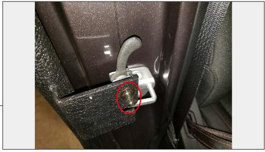
Loosely install the door latch using the M6x1.0x25mm bolts, flat washers, and lock washers.
