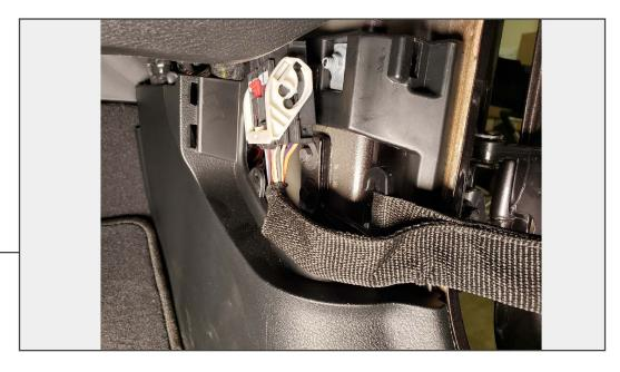
Roll down the windows so that the door is easier to handle while removing it from the vehicle. Unplug the door harness connector from the chassis harness (Slide the Red lock upwards, then hinge the white connector upwards). Slide the hinge strap off the chassis mounting hook.
