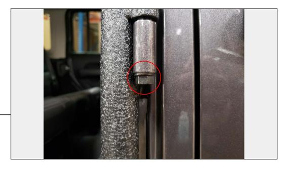
Install the new door to the vehicle hinges. It may be necessary to use a rubber mallet to seat the door all the way onto the hinge. Use the supplied M8 nut and washer to secure the door to the hinge.
