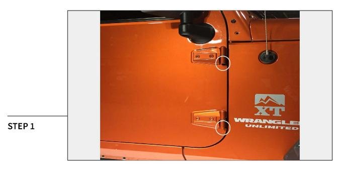
Begin by removing the T-50 Torx nuts on the bottom of the factory door hinges. These will not be reused.
