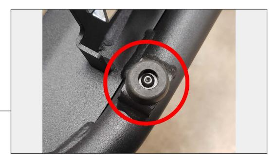
Install the rubber door stopper to the door using the M4x0.7x15mm screw, and M4 flat washer.
