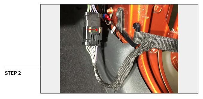
Roll down the windows so that the door is easier to handle while removing it from the vehicle. Access the door's electrical connector by tracing it under the dash. Unlock the red locking mechanism and then unplug the connector. Slide the hinge strap off the chassis mount. Lift the door up to remove it from the vehicle.
