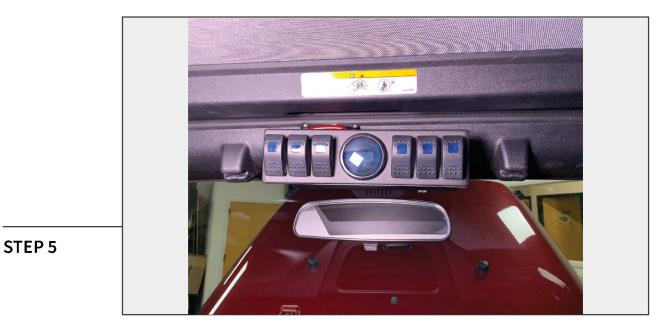
Route the plug from the Control Box through the firewall, up the A-pillar. Mount the Switch Panel over the rear view mirror. Using the attached bracket, clamp the bracket over sail panel hook.
