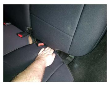
**Step 9\\ Rear Seats**Insert the lower passenger and driver side seat covers. Tuck the buckles in-between the upper and lower seat section.
