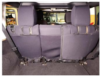
**Step 10\\ Rear Seats**From the back of the rear seats, pull the buckles from the lower seat cover and tuck under the seat.
