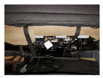
**Step 11\\ Rear Seats**From underneath the seat, connect the front to back straps to the buckles. Pull tight on the strap to secure the cover to the lower seats.
