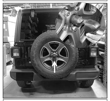
Step 1. Using a T-40 torx bit locate and remove the plastic lock from the backup camera as shown. Set factory plastic lock aside in a protected area.
