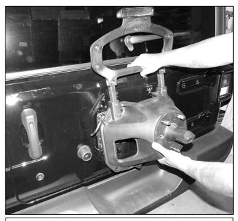
Step 6. Remove factory tire carrier from vehicle. Set factory tire carrier aside in a protected area.
