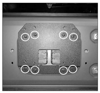
Step 2. Reinstall all 8 factory bolts through the hole in the relocation bracket and onto the vehicle as shown.
