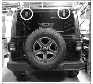
Step 1. Using a flat head screwdriver locate and remove factory window hinge cover as shown above. Set aside for later use.
