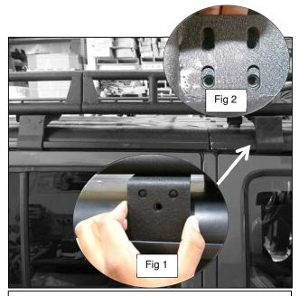
Step 3. Place supplied large mounting brackets towards the front of the Jeep as shown above fig 1. Line up the top mounting holes with the roof rack mounting holes as shown in fig 2.
