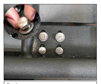
Step 4. Working on the top side of the large mounting bracket. Place a supplied M8x1.25x25mm hex head bolt with supplied M8 flat washer through the holes in the roof rack onto the holes on the mounting bracket. Tighten down using a 13mm socket. Repeat step for remaining bolts. Repeat step for 1-2 for remaining rear mounting brackets. Repeat step 1-2 for other side.
