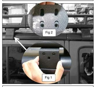
Step 1. Place supplied small mounting brackets towards the rear of the Jeep as shown above fig 1. Line up the top mounting holes with the roof rack mounting holes as shown in fig 2.
