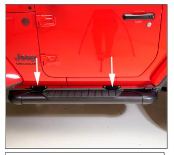
Step 4. Repeat step 1-3 for remaining running board brackets.
