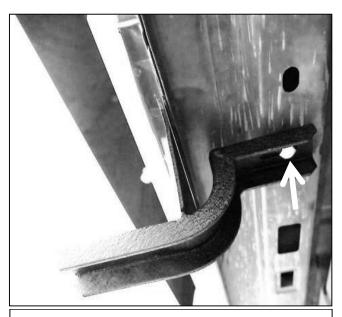
Step 2. Place a supplied M8x1.25x25mm hex head bolt (E) with supplied M8 large flat washer (F) through the holes in the mounting bracket hole and onto the vehicle. Tighten down using a 13mm socket.
