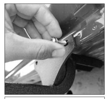
Step 3. Place a supplied M8x1.25x25mm button head bolt (B) with supplied M8 large flat washer (F) through the holes in the mounting bracket hole and onto the vehicle. Place a supplied M8 flat washer (C) at the end of bolt. Start a supplied M8x1.25 flange nut (D) at the end of bolt. Tighten down using a 13mm socket. Repeat step for remaining button head bolt.
