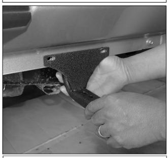
Step 1. Working towards the front of the vehicle locate and place supplied a L bracket (A) onto the vehicle as shown. Line up the holes in the L bracket with the holes on the vehicle.
