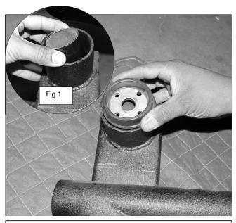
Step 2. Working towards the front mounting point (use step 1 as a reference) of the supplied rocker slider (A). Place supplied spacer (E) into the front mounting cup fig 1. Reinstall previously removed factory washer as shown.
