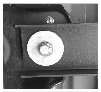
Step 5. Working towards the rear of the vehicle. Reinstall the previously removed factory bolts. Finger tighten only. Repeat step for remaining factory bolt. Tighten down all hardware using a 18m socket.
