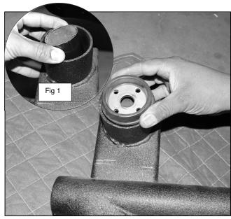
Step 2. Working towards the front mounting point (1) (use step 1 as a reference) of the supplied rocker slider (A). Place supplied spacer (E) into the front mounting cup fig 1. Reinstall previously removed factory washer as shown.
