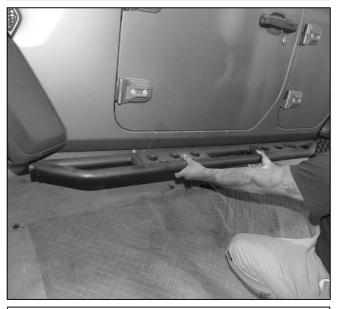
Step 3. With help from an assistant place supplied rock slider (A) onto vehicle. Line up the holes in rock slider with the vehicle hole. Push rock slider into position.
