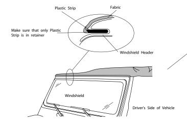
Note: For best possible installation, check to make sure that the soft top is perfectly centered on the vehicle.
