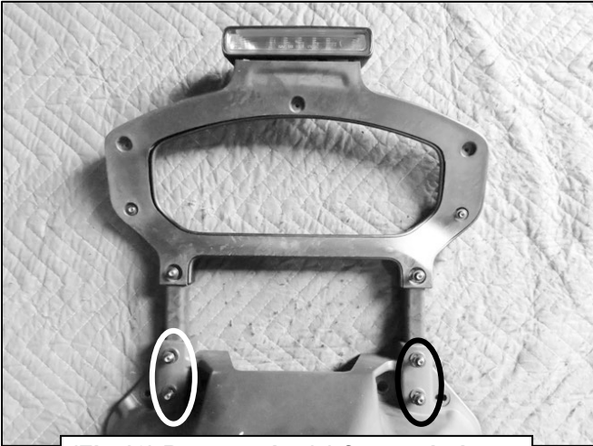
(Fig 10) Remove the (4) factory bolts to detach the main body of the spare tire carrier from the top CHMSL assembly
