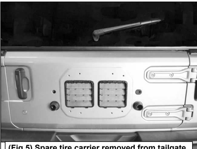
(Fig 5) Spare tire carrier removed from tailgate
