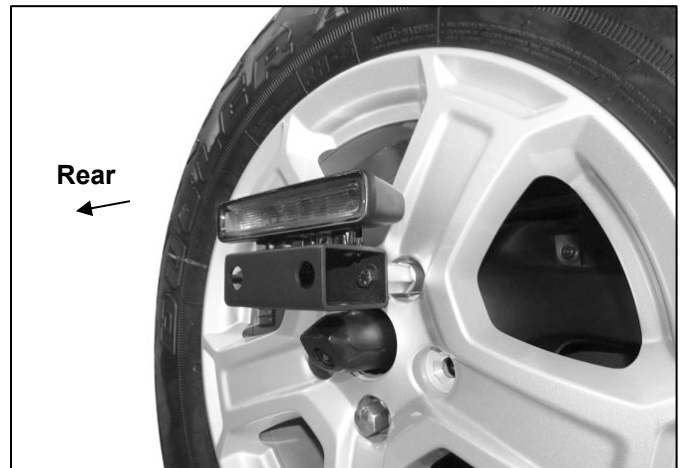
(Fig 18) Reuse the (2) factory bolts to attach the light to the top of the Bracket
