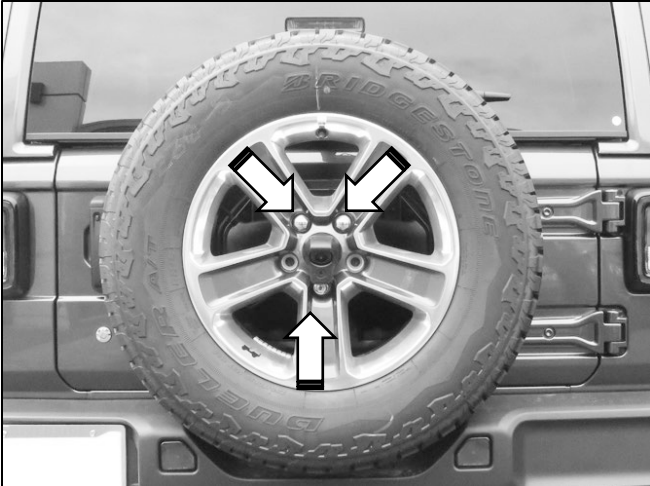
(Fig 1) Remove the (3) factory lug nuts to remove the Spare Tire from the back of the vehicle
