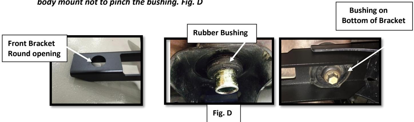
**Step 5:** Tighten all hardware to factory specs starting with the center bracket then front and rear.
