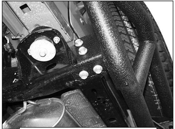
(Fig 9) Reuse factory hex bolts to attach Bumper to frame (driver/left side)
