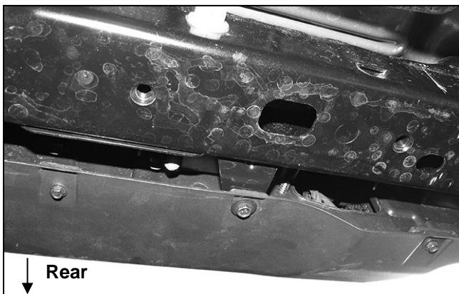
(Fig 3) Remove (2) hex bolts (if equipped) attaching bottom of bumper to cross member
