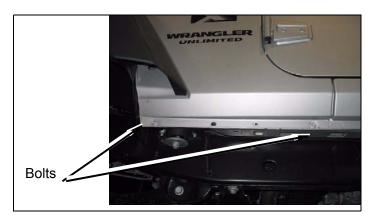
**b.** Cut off two weld nuts on back of body seam.
