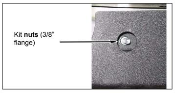
e. 4 Door Model: Tighten kit nut (3/8" flange) on kit bolt (3/8" x 2.0" carriage) on side of kit rocker panel.
