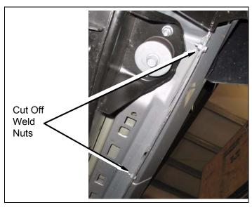
c. 2 Door Model: Position driver side kit rocker panel on vehicle. Mark and center punch last mounting hole on body seam using rocker panel as template.
