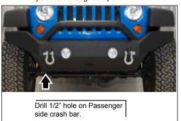
**c.** Install four *kit* **bolts** (1/2" x 1 1/4" Button Head) with **large thick washer** and **flange nut** through outer holes on bottom of bumper.
