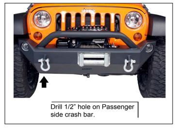
c. Install four *kit* **bolts** (1/2" x 1 1/4" Button Head) with **large thick washer** and **flange nut** through outer holes on bottom of bumper.
