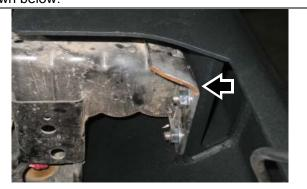
Remove small section of frame horn as shown in image above
