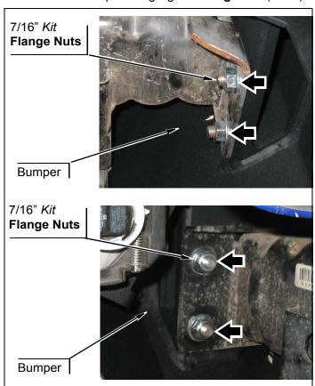
b. Note: 2010 - 2016 Models mark and drill passenger side lower crash bar. Mark and drill (using a 1/2" drill bit) passenger side lower crash bar so kit bolts (1/2-13 x 1 1/4" button head) may install through bumper & crash bar.
