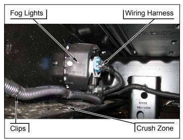
**4.** Remove four nuts, four spacer plates and front bumper from frame horns.
