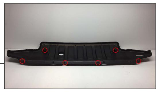
Using a flat head screwdriver or trim panel removal tool, remove the (6) plastic push pins securing the factory splash shield to the vehicle. (4) Across the front edge, (2) on the rear edge.
