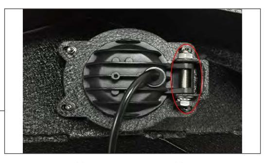
**OPTIONAL LED FOG LIGHTS:** Install the (2) fog light brackets using the (8) M4 bolts, lock washers, flat washers, and nuts. Install the (2) LED fog lights to the brackets by using the (2) M8x1.75x50mm bolts, lock washers, flat washers, and nuts.
