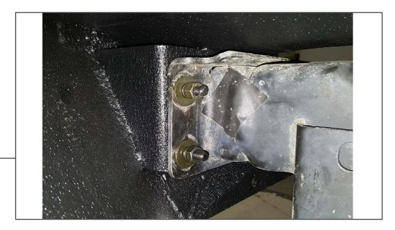
Install the bumper by using the (4) M10 nuts, (4) M10 x 25mm bolts, (8) lock washers, and (8) flat washers to the vehicle. Torque to 40 lb ft.
