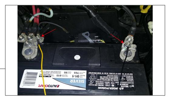
**OPTIONAL FOG LIGHT WIRING:** Install the yellow 12+ volt wire to the positive battery terminal. Connect the black ground wire to the negative battery terminal. Secure any extra wire out of the way.
