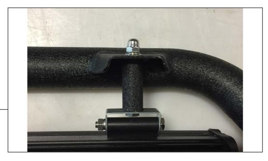
**OPTIONAL LIGHT BAR INSTALLATION:** Begin by installing the 70mm bolt through the silver light bracket. Install the bracket to the light bar using (1) M8 x 1.25 x 60mm bolts, flat washers, lock washers and nuts for each side. Slide the light bar bracket spacer onto the 70mm long bolt. Install the light bar to the bumper using the flat washer, lock washers, and nuts.
