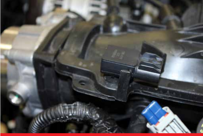
E. Install supplied 3bar map sensor using provided harness adaptor.
