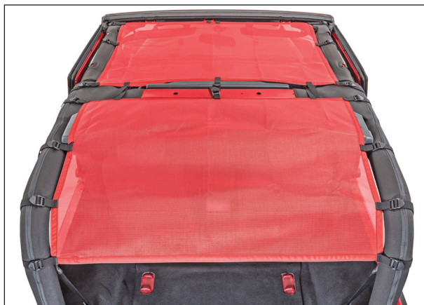
Rear Cargo Area Mesh Top Shown for 2007-2017 2 Door Wrangler with Bimini Mesh Top.
