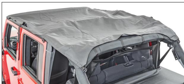
Shown: 4-Door Version Header in place with the fabric portion extending back towards the rear of the vehicle.
