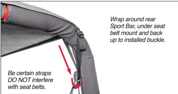
**Step 7** (all Bimini Plus for 4-Door) Secure rear/side straps. Locate the side strap positioned on the end of the top and wrap the strap around the rear Sport Bar hoop, under the seat belt mount and back up to the buckle. Pull tight. Repeat on opposite side. Make sure all straps are tight and secure.
