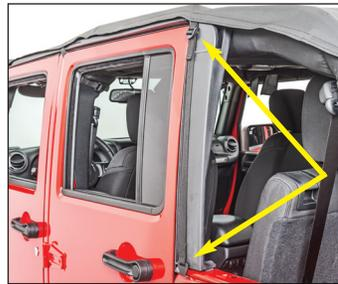
**Step 6** (Bimini Plus for 4-Door) Install Side Tension Straps. Thread Side Tension straps through the buckle on side of the Bimini Plus. Hook end of the strap under the belt rail and slide it under the door surround. Pull the strap tight. Repeat on opposite side
