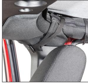
**Step 4** (4-Door) Install Side Tension Straps. Thread Side Tension straps through the buckle on side of the Bimini Plus. Hook end of the strap under the belt rail and slide it under the door surround. Pull the strap tight. Repeat on opposite side of vehicle.
