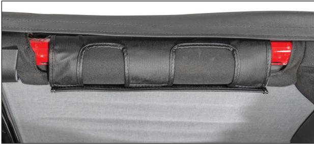
**Step 5** (Bimini Plus for 4-Door) Secure side straps onto Horizontal sport bars. Wrap the flap above the door opening around the horizontal sport bar and then fasten the hook and loop closure. Repeat on both sides of the vehicle.
