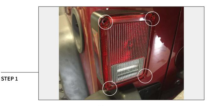
Using a Phillips head screw driver, remove the (4) screws on the tail light.
