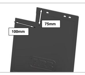
15. IF FITTING MUD FLAPS (ARB SHOWN part no: 3500370). Cut a section out of each opposite corner of the mud flap as shown.
