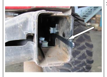
7. Place M12 cage nuts in cage nut plate and slide into chassis rail so bottom two cage nuts line up with the two forward most holes on underside of chassis. Check that bottom holes line up with cage nuts correctly. If the chassis holes are slightly off use a die-grinder to correct. RH side shown, repeat for left hand side.
