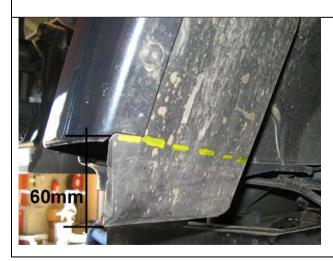
3. The plastic inner guards can now be trimmed. Measure 60mm up from the bottom edge of the inner guard and draw a horizontal line as shown.
