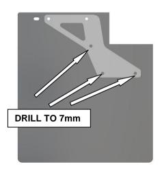
Place mounting panel on flap as shown lining up the two inner mounting holes on the mud flap. Mark and drill holes as shown to 7mm. Once complete place on vehicle and secure using black M6 hardware.
