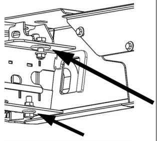
9. Drill pinning bolt using a DIA 10.0 drill bit. Clean away any debris and paint bare metal using a rust preventative coating.
