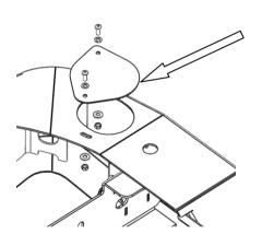
Fit carrier cover panel to bar using 2 x M6 x 16 button head SS screws, SS flat washers, ZP flat washers and nyloc nuts. Place Stainless Steel hardware on top of the cover plate as shown.
