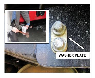
8. Place bar onto chassis and secure to captive nuts using M10 x 50mm bolts, spring washers and washer plates. Leave bolts finger tight. Secure all other points using M12 x 40mm bolts, spring washers and flat washers. Torque to specification.
