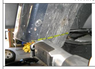
4. Cut along the marked line being careful not to damage the flared guard.
