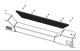
5. Fit centre cover panel to bar using 5 x M6 x 20 bolts, spring washers, flat washers and flange nuts. Place bolt head towards the front of the vehicle.
