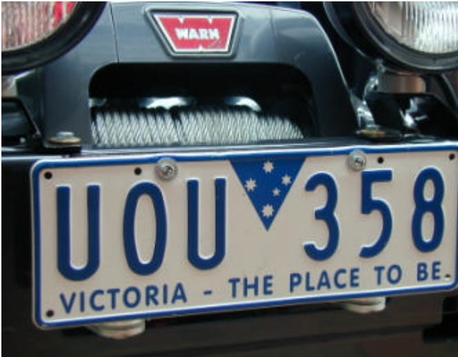
Bolt number plate to number plate bracket using 6mm hardware.
