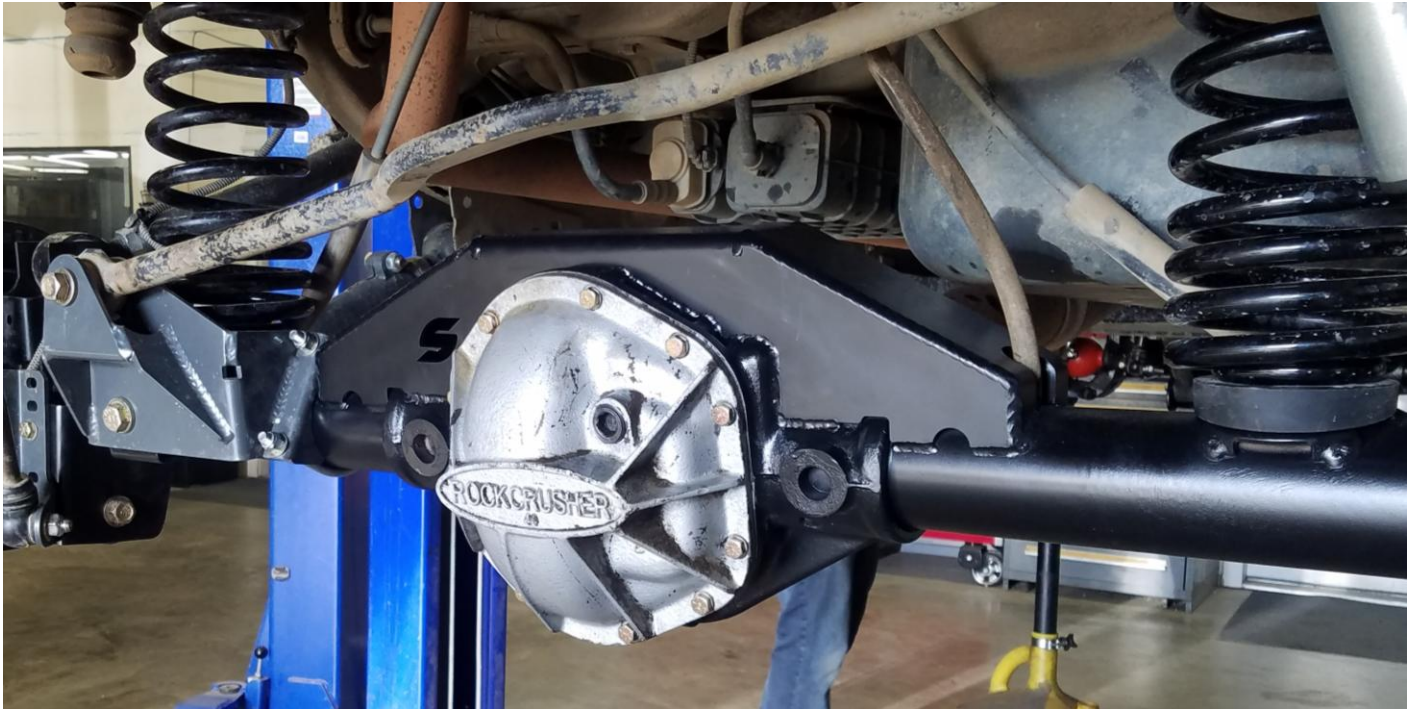
Figure 7. Completed and Painted Rear Truss
