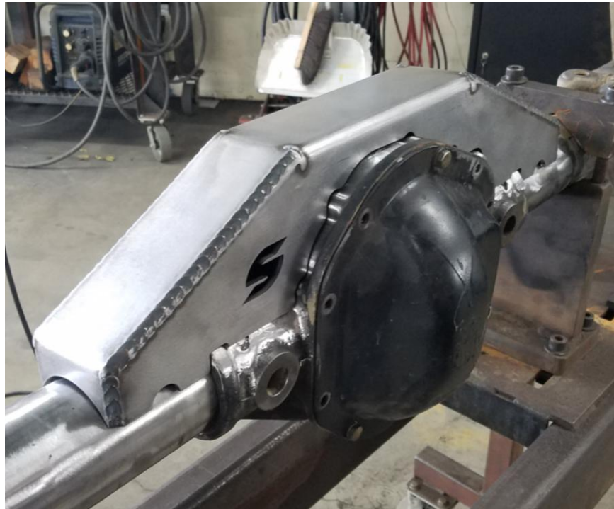
Figure 6. Truss Correctly Placed On Axle Housing
