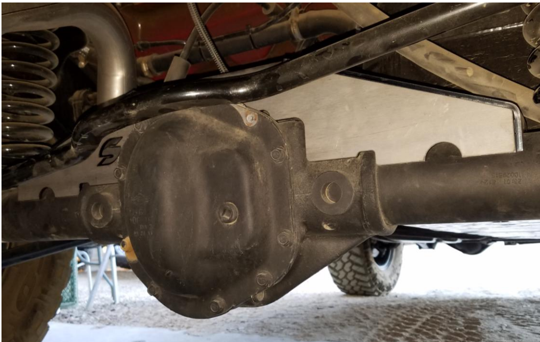
Figure 1. Truss Placed on Axle
