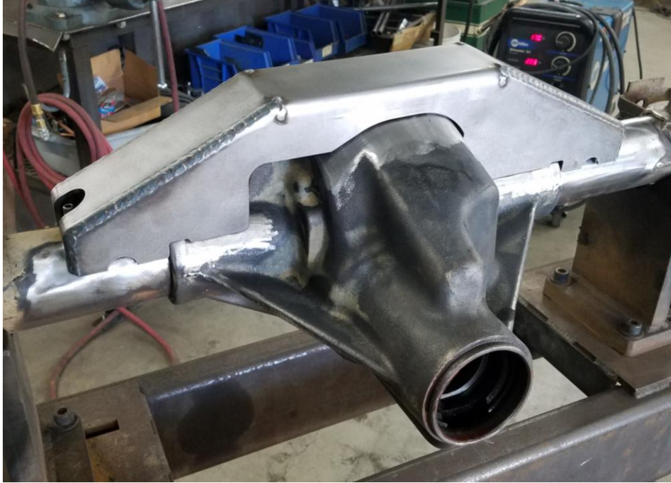
Figure 5. Truss Correctly Placed On Axle Housing
