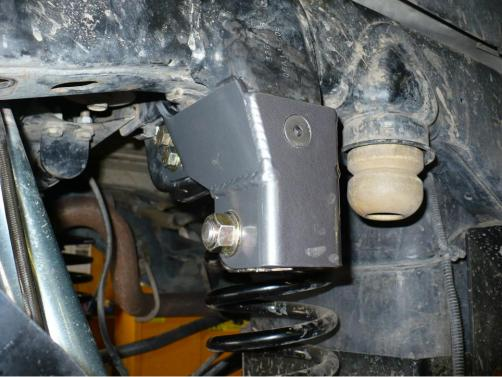
9) Reinstall rear tire and lower vehicle to the ground. Connect TB and new TB bolt and torque to 125 ftlbs.
