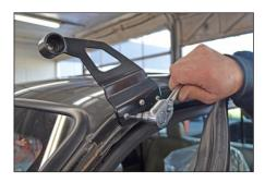
**STEP 9** - Install the 1/4-20 x 3/4" stainless steel button head bolts. Snug bolts, but do not fully tighten.
