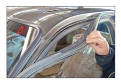
Step 1 - Beginning with the driver side door, remove the door seal in the top front area of the door.
