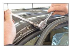
**STEP 7** - Use provided Grip-Sert tool to fasten nut by tightening down the bolt while placing wrench on center nut. Do not let nut turn when tightening. Repeat steps 1 thru 7 on passenger side door.
