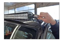
**STEP 13** - Fasten KC LED light to driver side bracket. Adjust bar until level and tighten all bolts.
