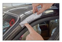
**Step 2** - Place the template in the base of the rain gutter, lining up the A-pillar and roof seam marks.
