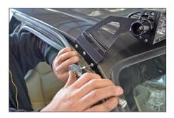
**STEP 12** - Align passenger side bracket with light bar over Grip-Sert holes and install bolts.
