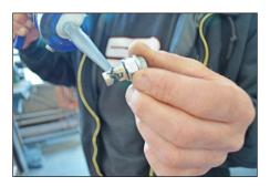
Step 5 - We recommend applying a small amount of silicone to the splined area of the Grip-Sert.
