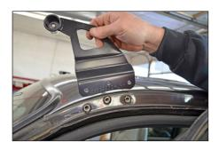
**STEP 8** - Install driver side bracket with the point facing forward.
