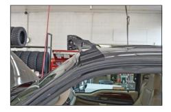
**STEP 15** - Place rubber seal back into the drip rail. This will protect the bracket and wiring from the elements.
