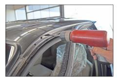
**Step 4** - Drill marked holes with a 5/64" pilot drill bit and then slowly step up to a 3/8" drill bit.
