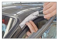
Step 3 - Mark the holes with a center punch over the template.
