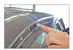
Step 6 - Insert supplied Grip-Sert rivet nut into holes flush with the metal surface.
