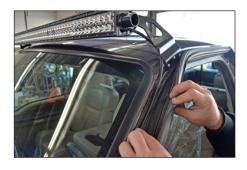
**STEP 14** - Route the power wire down the A-pillar under door seal and wire the light bar as noted in the light bar instructions.
