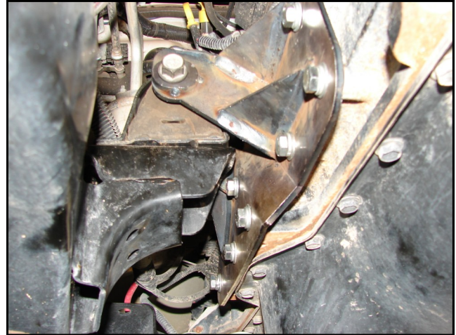
PS Block Bracket Installed
