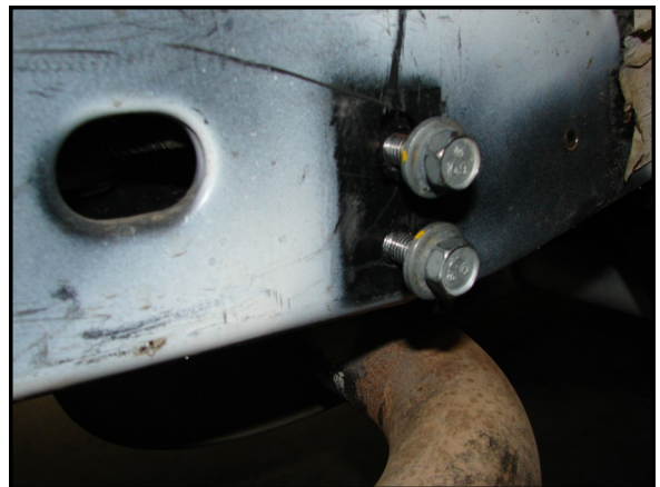
2– Factory bolts per side of frame.
