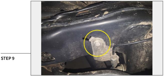
Remove (1) brake line mounting bolt on the frame of the vehicle.
