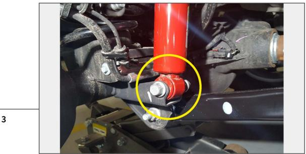
Remove the lower shock absorber bolt from the axle mount. Hardware will be resued.
