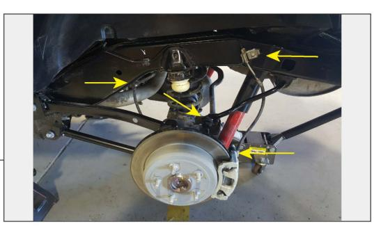
Re-install the rear shock absorber to the axle mount using original hardware. Re-install the rear sway bar link to the sway bar reusing original hardware. Re-install the brake line bracket and the wiring harnesses to the frame rail at the original locations.
