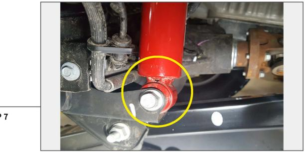
Re-install the shock absorber to the axle using the original hardware.
