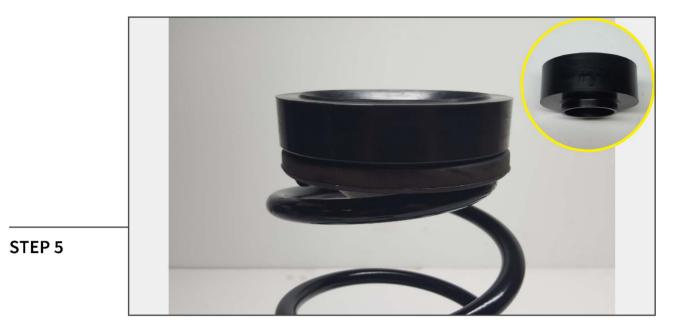
Install the coil spring spacer over the factory bump stop on the vehicle, ensuring the spacer lip is facing downwards. Install the coil spring with the original coil spring isolator on the top of the spring. Repeat this procedure to the opposite side of the vehicle.
