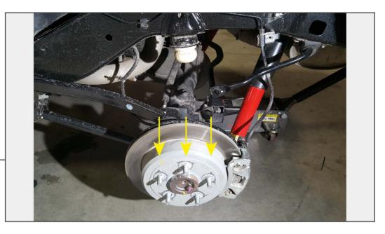
Press downwards on the axle to allow the spring to become loose. Remove the spring and spring isolator from the vehicle. Repeat this procedure to the opposite side of the vehicle.
