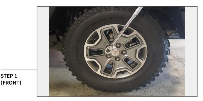
Safely lift and support the front of the vehicle in the air using a jack and jack stands. Remove the front wheels from the vehicle.
