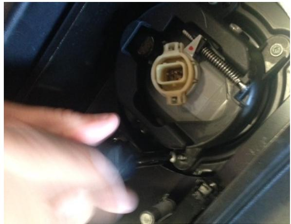
F) Line up the light housing to the tabs on your new bumper as shown and push the plastic fasteners through from the opposite side with the small ridged end of the fastener coming towards you.
