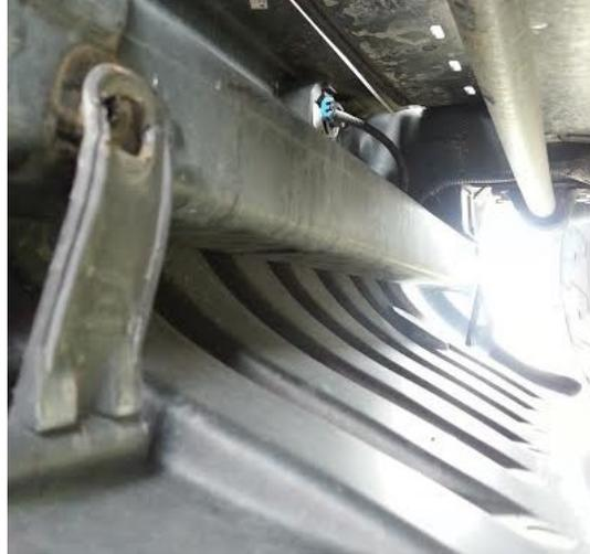
B) Remove the factory front bumper by re-moving the 4 factory nuts on both bumper mounts. Unclip the wiring harness from the fog lights.
