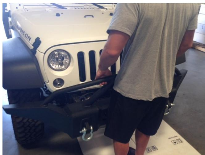
B) Loosely insert the lock washers and nuts onto the studs. Once all studs are in the proper mounting positions check the alignment and tighten to 60 ft/ lbs .
