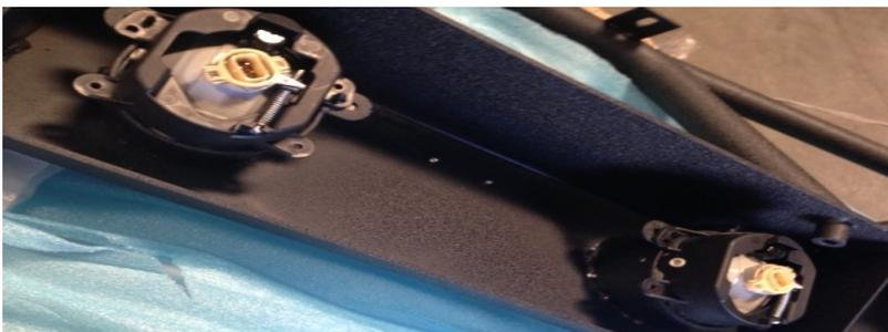
2) Locate the mounting plates and studs on the inside of the bumper. Also locate the 8 nuts and lock washers provided with the hardware.
