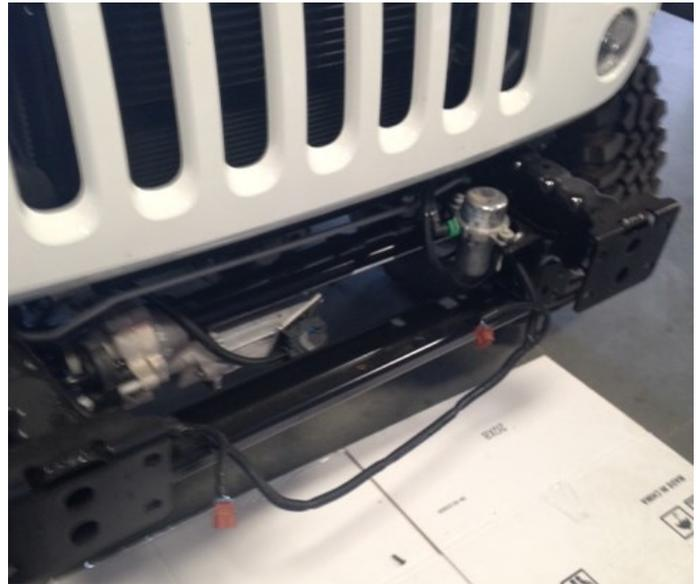
E) Remove the factory fog lights from the bumper for re-use on your new bumper by removing the 4 screws holding each one in place. (Not applicable on all models, only the ones with cut outs for the fog lights, if you don't have factory fog lights or compatible bumper skip steps D-F)
