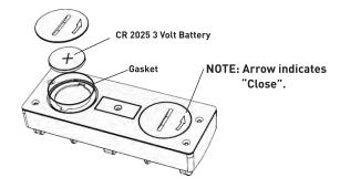
Install the Cr2025 batteries as shown. Be sure to turn the battery door to the right (clockwise) to open, the arrows indicate the direction to close (counter clockwise).
