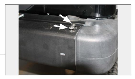
Remove the (2) T27 screws that secure the plastic caps on each end of the bumper.
