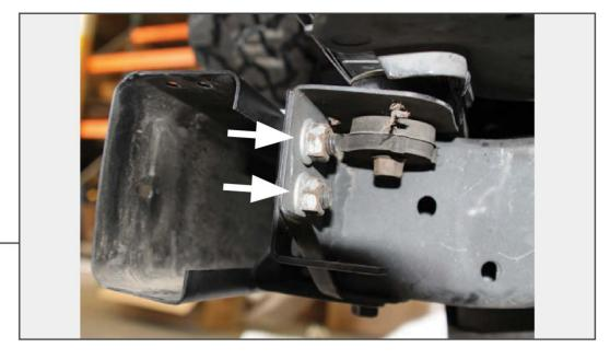
Once you remove the plastic end caps, there will be (2) 18mm nuts that attach the bumper to the frame. Remove these nuts on both sides and remove the bumper from the vehicle.
