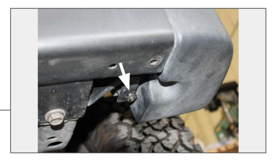
Remove the remaining T27 screw securing the plastic cap to the bumper.
