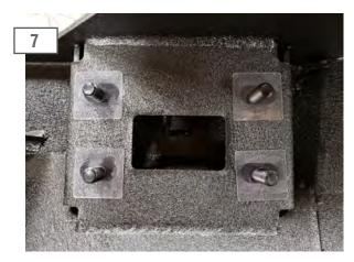
Insert the (2) dual bolt plates through the back side of the bumper mount and secure using the plastic holders.
