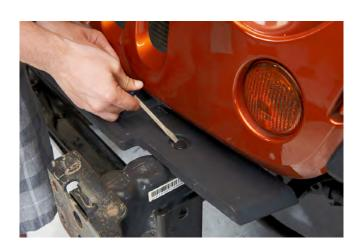
**STEP 3** // Remove the 2 push pins holding the top cover onto the vehicle
