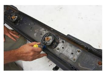
**STEP 4** // To remove the fog lights, loosen the 4 phillips screws on each light.
