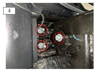
From under the vehicle, access and remove the (8) 18mm nuts, and (4) 18mm bolts securing the factory bumper to the vehicle. Then fully remove the bumper from the vehicle.
