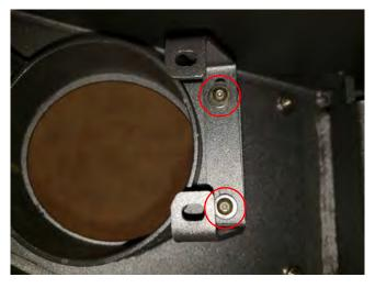
**STEP 5** // Install the (2) LED Fog Light Brackets to the fog light mounts of the bumper using the (4) M6 torx bolts, washers, and nuts.
