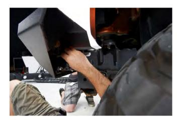
**STEP 7** // Slide bumper into place, and secure using the supplied hardware.
