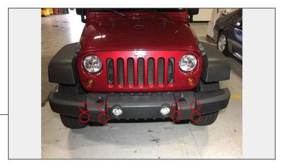
From under the vehicle access and remove the (8) 18mm nuts securing the factory bumper to the vehicle.
