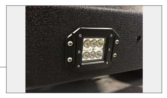
Remove the center block off plates to install the flush mounted bumper lights. The Allen bolts will be reused.
