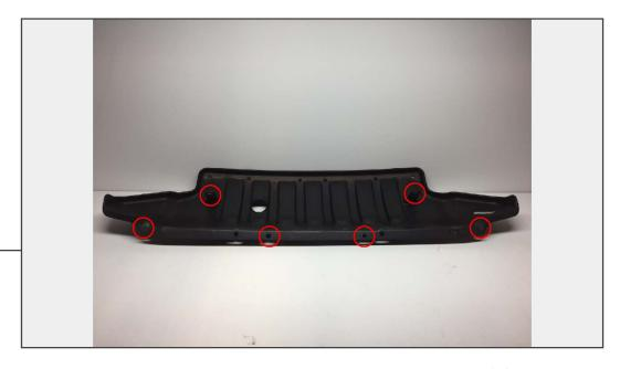
Remove the (6) plastic push pins securing the factory splash shield to the vehicle. (4) Across the front edge, (2) on the rear edge.
