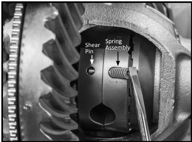
Figure 7: Install spring assemblies in holes
