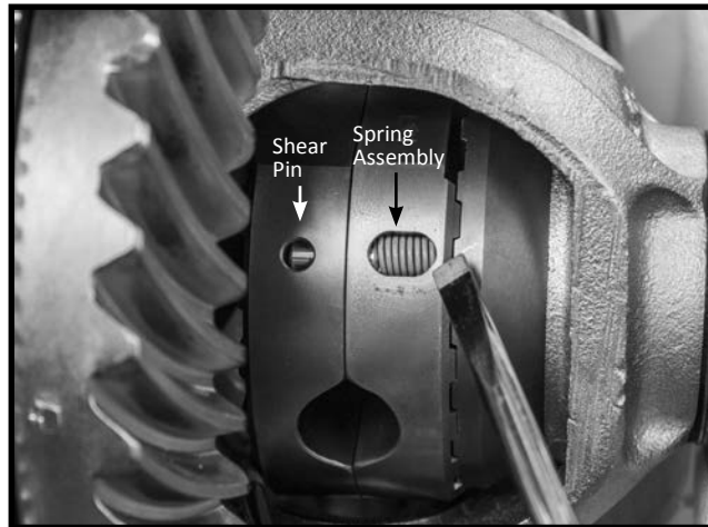
Figure 8: Snap spring assembly into hole
