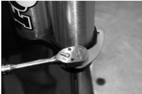
Fig. 8: Spanner wrench tighten
