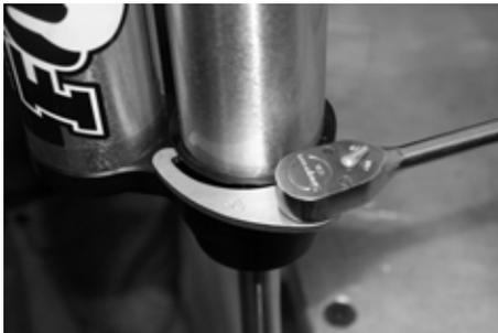
Fig. 7: Spanner wrench loosen
