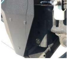
Failure to secure the winch plate to the frame with the bolts provided will cause winch plate to twist and cause your winch to malfunction.
