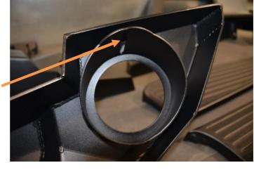
If the light has a grill, position the grill between the light and the inside of bumper.
