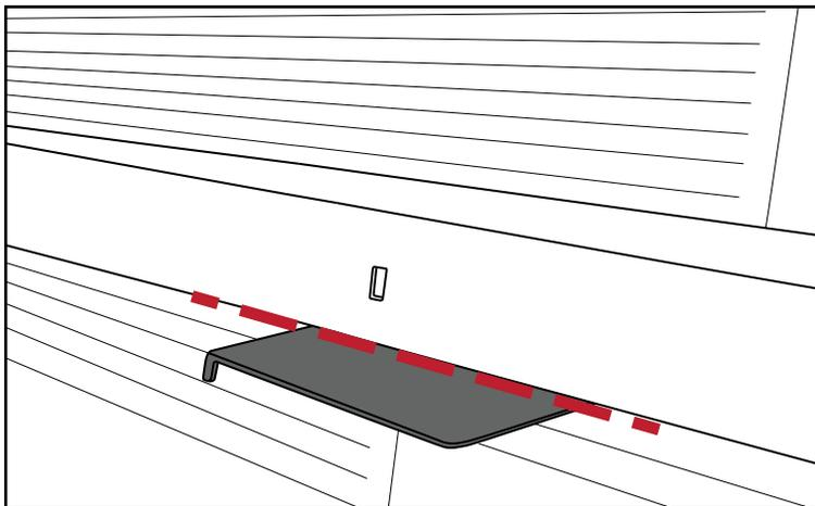
8. Flip sensor 180° from original position and reinstall using rectangular center pin.
