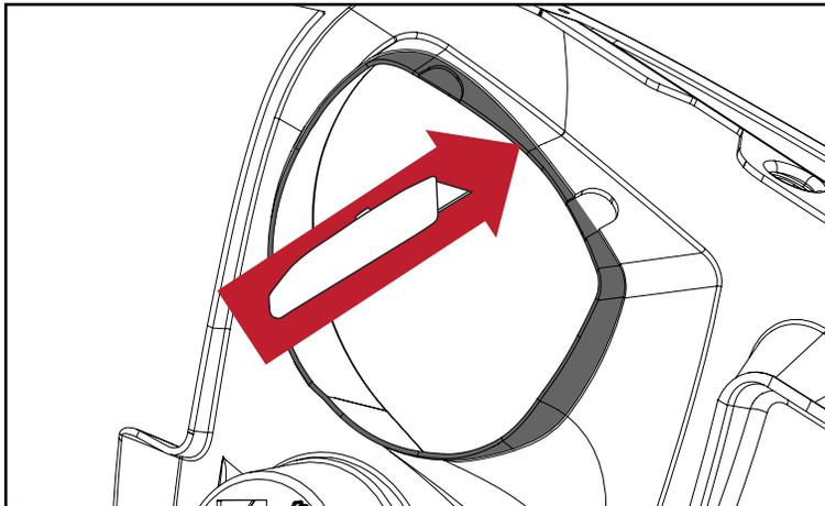
11. Install factory turn signal housing into Spartan Grille. Repeat for opposite side.
