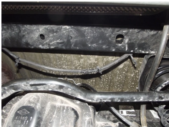
Photo 1 – Horizontal beam with wiring harness clips removed
