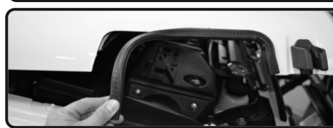
6. Using the crosshairs on the cutting template as a guide, use a 1 3/4" hole saw and drill out the two holes on the template. Make sure you drill past the second layer of the hood. Please use caution!!!
