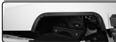
10. Place the 16" vinyl trim onto the edge of the cut out. Re-install your hood and the snorkel is ready for installation
