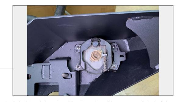
Using (4) M4 Allen bolts, (4) M4 lock washers, (4) M4 flat washers, (4) M4 nuts, attach the fog light to the bumper and bracket installed in Step 5. Repeat for both fog lights.
