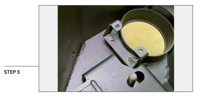
Using (2) M4 bolts, (2) M4 lock washers, and (2) M4 flat washers, attach the fog light bracket to the bumper. Repeat on both sides of the bumper.
