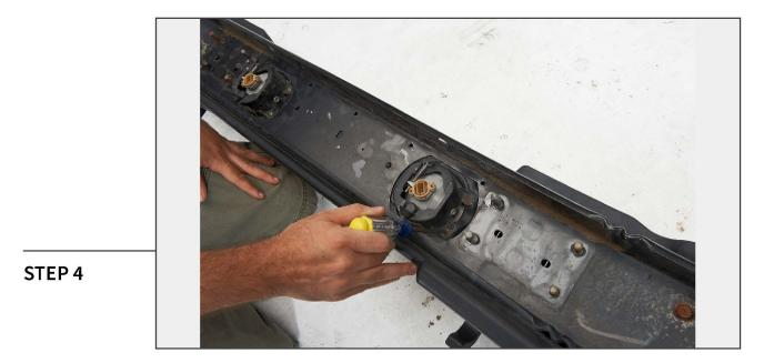
Remove the fog lights by removing the (4) Phillips screws on each light.
