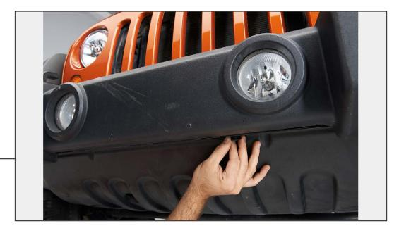
Using a flat head screwdriver or trim panel removal tool, remove the 6 pins holding the splash guard onto the vehicle.
