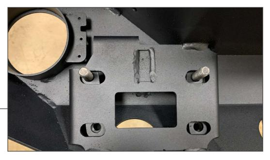
Place the nut/bolt plates behind the bumper mounting pad. This will allow for minor adjustment side to side.
