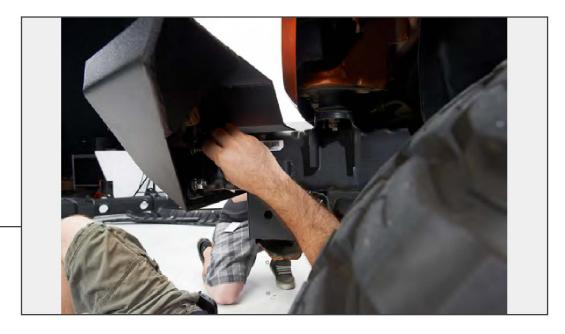
With help, carefully install the bumper. Secure the bumper to the vehicle using the provided M12 hardware. Reconnect the fog lights (extending the wiring may be required). Installation is now complete.
