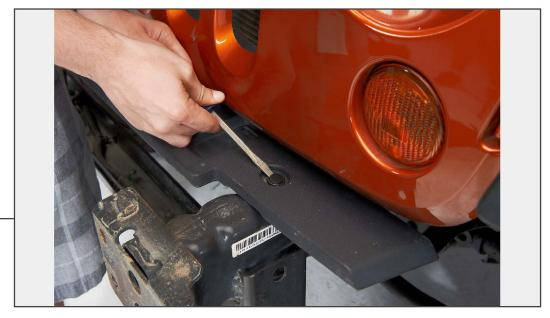
Using a flat head screwdriver, remove the 2 push pins holding the top cover onto the vehicle.
