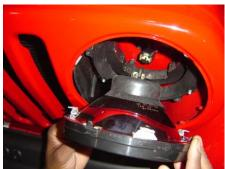
NOTE: When installing be sure rubber boot is snugly fitting over the reflector providing a good seal against moisture. In the event any moisture is trapped inside the headlight causing it to steam up, please follow these procedures: Peel back the rubber boot and carefully remove the bulb by releasing first the bulb spring. Allow vapor to escape by holding the headlight in sunlight or using a hair dryer. When completed, assemble the bulb and re-seal the boot around the reflector.
