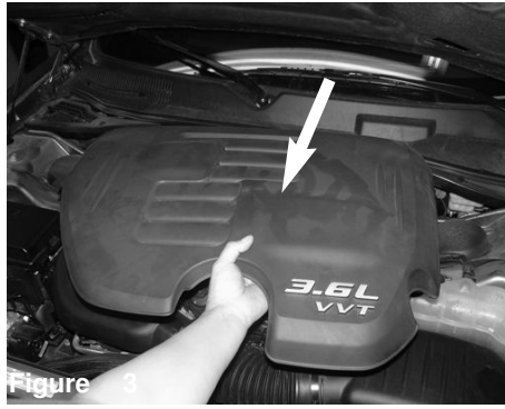
Figure 3 Lift up and detach the engine cover from the engine
