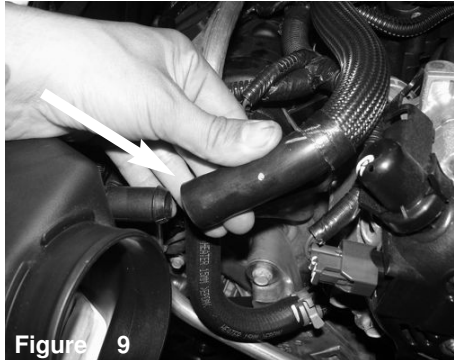
Figure 9 Pull back the crank case line from air box fitting.
