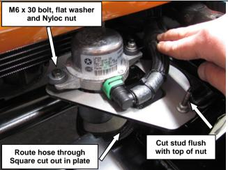
8. Un-bolt vacuum pump and place new mount on chassis as shown. Orientate pump as shown and mount using original nuts on studs and M6 x 30 bolt, flat washer and Nyloc nut on opposite rubber mount. Secure piping using cable ties in kit. NOTE: Cut stud flush with top of nut.
