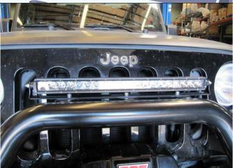
16. The top tube mount can be used for LED light bars or fitting of radio aerials.
