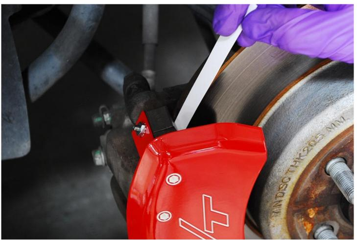
Use the included .013mm paper feeler gauge and verify clearance between the brake rotor and fastening clip. The feeler gauge should be able to slide in and out without obstruction.
