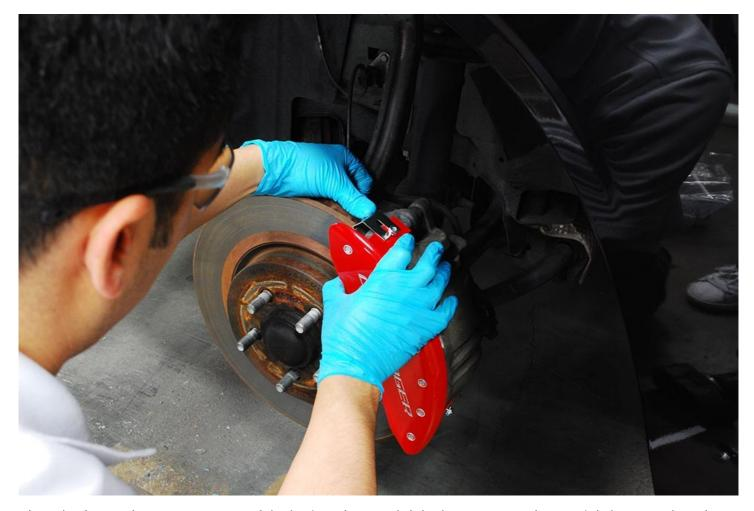
Place the front caliper cover on top of the brake caliper and slide the mounting clip on while keeping the caliper cover centered and snug against the face of the brake caliper.
