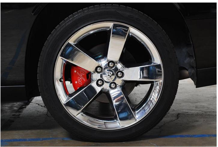
Reinstall the rear wheel. Be careful not to damage the caliper cover when installing the wheel. Verify that the wheel clears the caliper cover before lowering the vehicle. Tighten lug nuts per manufacturer's specifications using the torque wrench. Repeat for the brake caliper on the opposite side.
