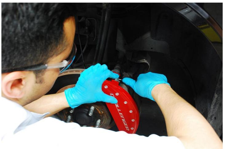
Tighten down the lock nuts with a 3/8 inch wrench to 25 inch-pounds (about 1/2 turn past finger tight).
