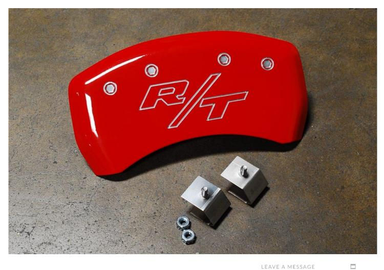
The fastening system for the rear set is engineered slightly different than the front. Before installing the fastening clips, remove the lock nuts and place them aside.
