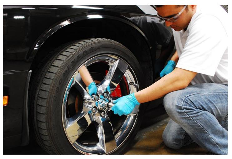
Remove Jack Stand(s) and lower vehicle. Tighten lug nuts per manufacturer's specifications using the torque wrench.
