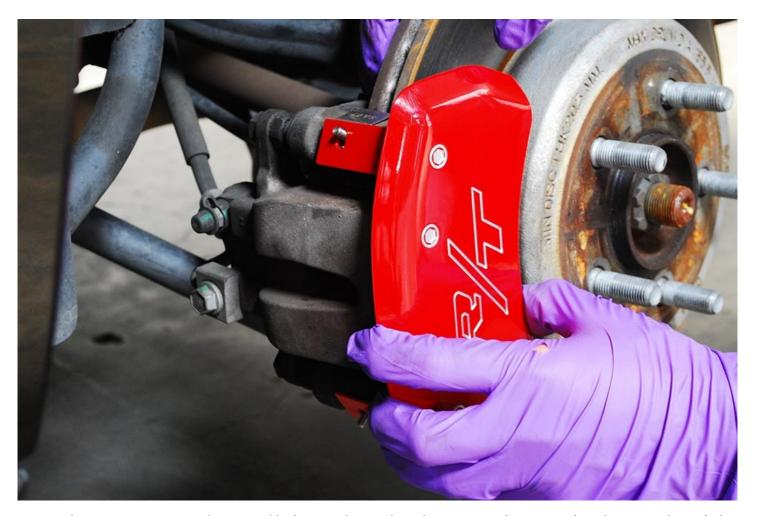
Rotate the cover to position the second hole over the stud on the opposite fastening clip. There may be a slight stretch involved when lining up the second stud. This is normal.
