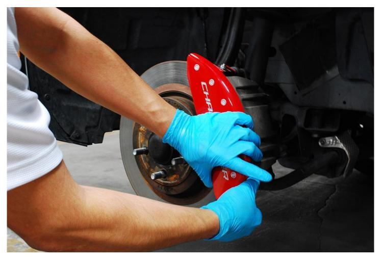
Make sure that the caliper cover is centered. Hand tighten the lock nuts.
