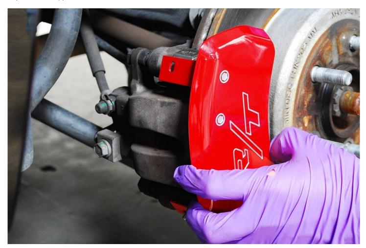
Place cover over rear brake caliper and position hole in the bridge over the threaded stud located on the fastening clip.
