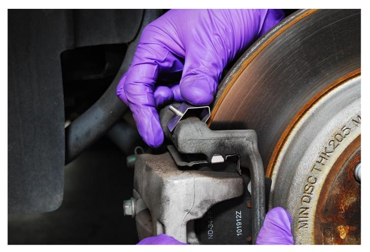
Slide fastening clip on to the rear caliper bracket as shown.
