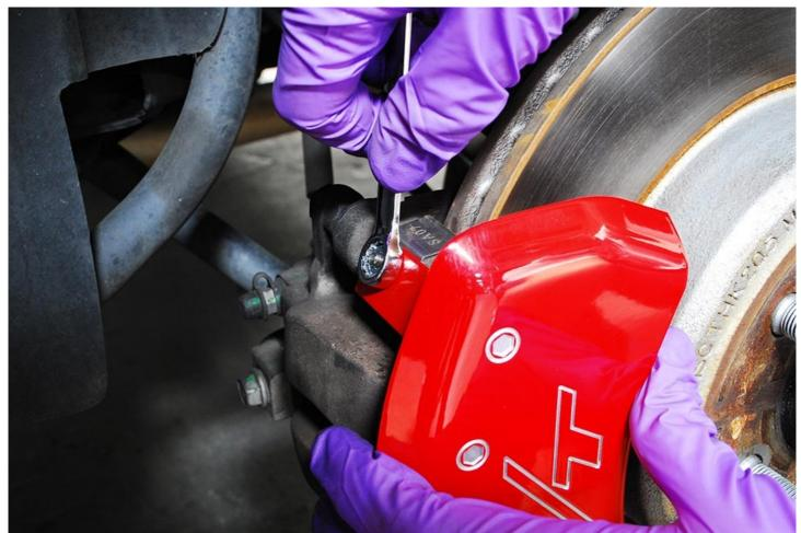
Reinstall the lock nuts that you previously removed off the fastening clips. Tighten down to 25-inch pounds (about  $\frac{1}{2}$  turn past finger tight).
