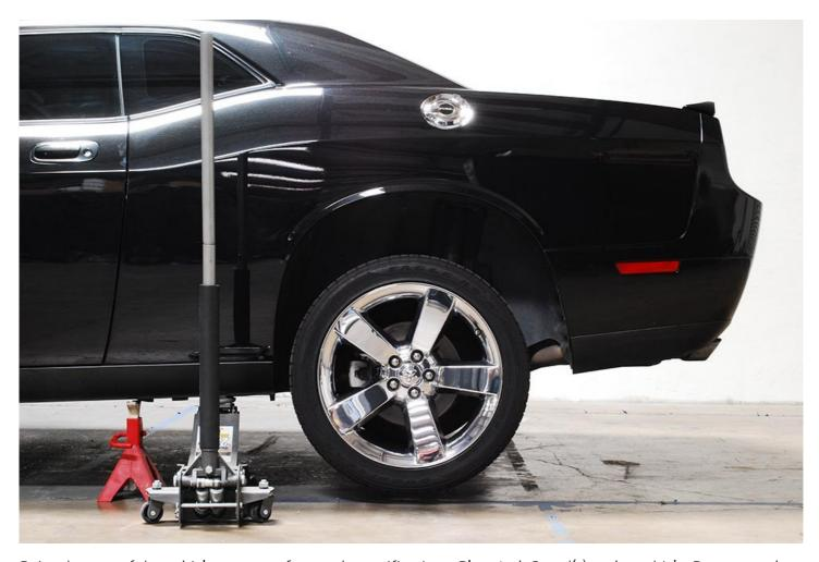
Raise the rear of the vehicle per manufacturer's specifications. Place Jack Stand(s) under vehicle. Do not conduct installation without Jack Stands in place!
