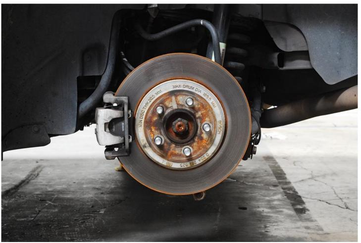
Remove the rear wheel with an Impact Wrench or Lug Wrench.
