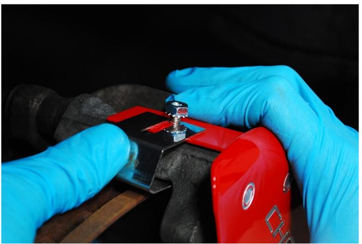
Be sure to slide the top of the clip underneath the fastening lock nut. The bottom side of the clip should slide in between the rotor and the caliper bracket.
