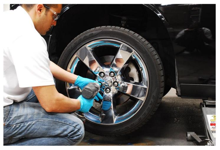
Remove the front wheel with an Impact Wrench or Lug Wrench.
